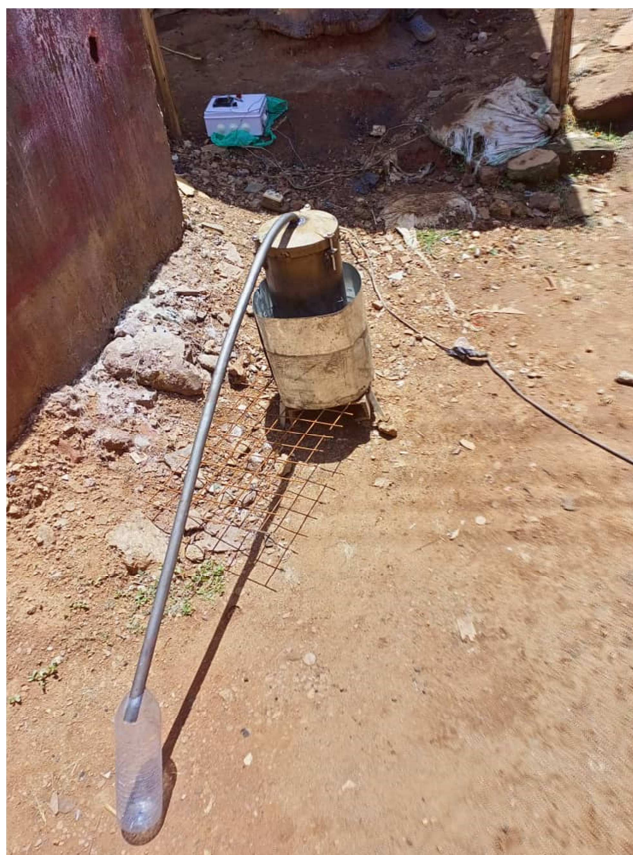
Figure 4. A complete setup of a pyrolysis reactor and a temperature-controlling system.
